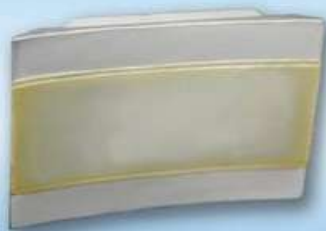
Asymmetrical Johansson Monochromator, R188, cut angle 10°59', LiF (220), 2d=0.284 nm
