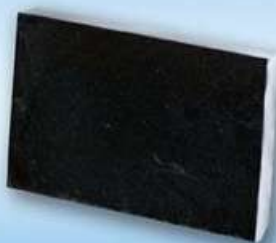
Flat monochromator. Graphite (0002), 2d= 0,668 nm
