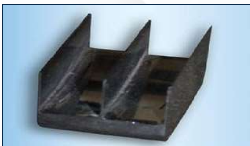
X-ray interferometer. Si(220), 2d=0,384\text{ nm}
