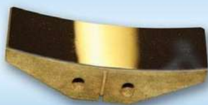
Johann cylindrical analyzer. InSb(111), 2d=0,748 nm
